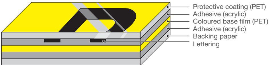
Brother laminated TZe labels consist of six layers of materials, resulting in a thin, extremely strong label. Characters are formed with a thermal transfer ink and sandwiched between two protective layers of PET (polyethylene film). The result is a virtually indestructible label that can withstand harsh conditions.
